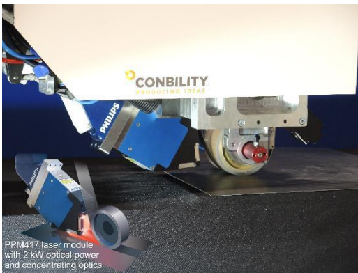
Fig. 3: VCSEL Tape Placement and Winding Applicator. Copyright: Conbility GmbH.
