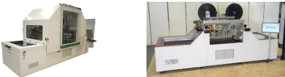
Fig. 1: “PrePro 2D“ machine system for tape placement of tailored blanks and laminates with in-situ consolidation. Copyright: Fraunhofer IPT.
