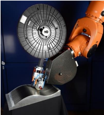
Fig. 2: "PrePro 3D" applicator for modular integration into existing production systems. Copyright: Fraunhofer IPT.
