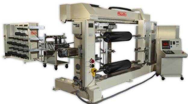
Picture 2: Filament Winding Machine Type 1: Roth Composite Machinery develops tailor-made plants for individual customer requirements. Copyright: Roth Composite Machinery.
