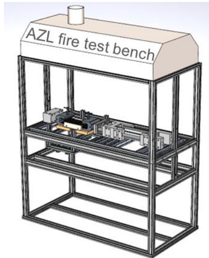
Figure 13: AZL Fire test set-up, for testing materials on strength under fire loading.
