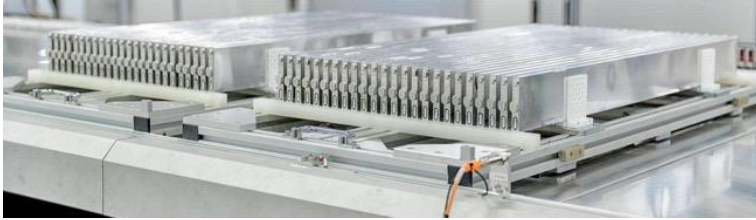
BYD blade cells, LFP type
